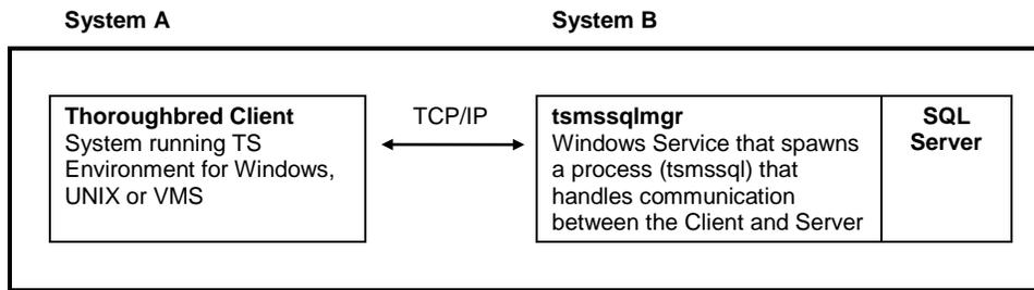
In the above figure the information is sent over the network to the server system. Once the requests reach the Server Process it creates SQL statements that are interpreted by the server system. The results are then passed back to the client through the Server Process.
