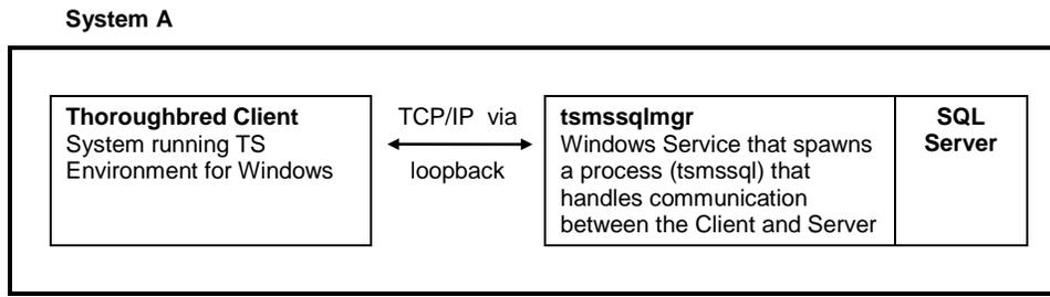
In the layout described by the above figure, the information is sent to the Server Process through the loopback TCP/IP address.
