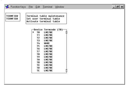
To select a device and terminal table to maintain, move the cursor over the selected device and terminal table and press **Enter**.
