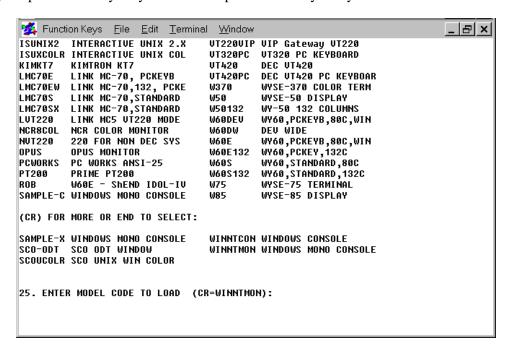
Each terminal table is identified by a model code. These model codes are displayed on the defined terminal table list screen along with the corresponding descriptions of the terminals.
