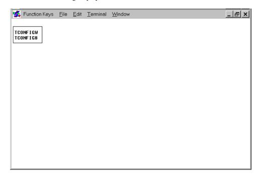
This window allows you to select either TCONFIG8 for non-windowed terminals or TCONFIGW for windowed terminals.
