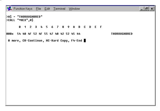
The \*HEX utility produced a hexadecimal dump to display contents of the A\$ string variable. The message line at the bottom of the listing displays a set of options that will prove useful when you have a very long string contained in a string variable.
